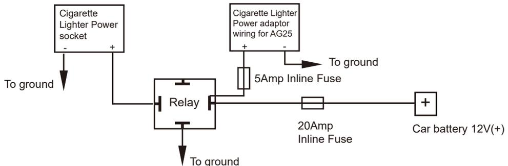
Note: The power connector can only be installed on a 12V cigarette lighter; it must be installed by an authorized dealer.
